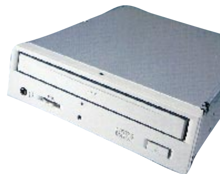
The Mitsumi FX-120 —one of the first 12-speed drives
